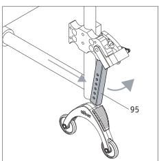
• Once the wheels are fitted, you can return the anti-tippers to their starting position. To do this, push the wheelchair forwards and push back the holding rod [95] using your foot at the same time.
