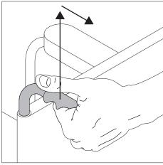
• While doing so, pull the wheelchair upwards and to the rear a little by its handles until the wheelchair has been raised and the anti-tippers click into a fixed position.
